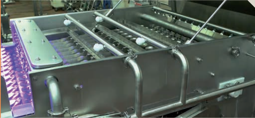
CIP spray balls and nozzles in the EBS 400
