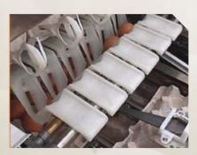
The Moba Prima 2000 is a reliable, economical no nonsense machine. A machine with a relatively low investment price enabling it to grow with your company needs in the future. The Prima 2000 is a stainless steel egg grading and packing machine with a capacity of 20,000 eggs/hour. By means of an Upgrade Kit, the Prima 2000 can be expanded to become a full Moba 2500 (30,000 eggs/hour).
